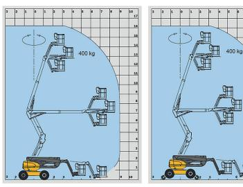
All dimensions in flat situation. Telescope arm will be blocked above 4,8° gradient in rail mode, maximum reach till 120 mm. cant is 8.65m, above 120 mm. cant the reach is 6.35m.
